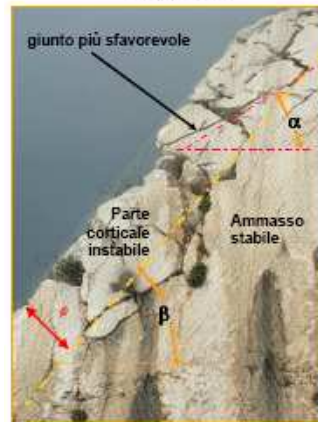
Diagram of a rock face with an indication of the main geometrical parameters
